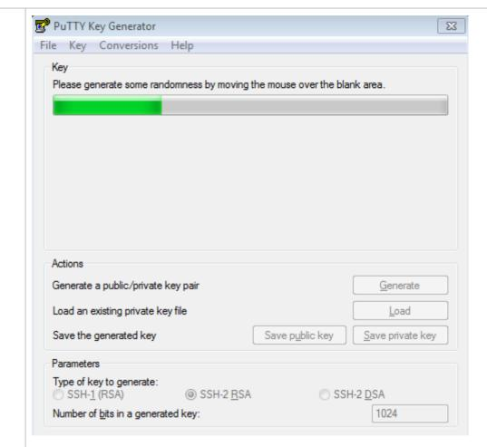
To ensure security of the RSA public key authentication, the length of the generated RSA key pair must be equal to or larger than 768 bits. In this example, the length is set to 1024 bits.
