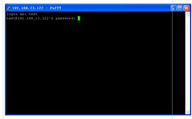
Type in the correct user name and password, and you can log in to the SSH terminal interface, as shown in Figure 14-11.
