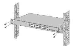
3. Place the switch in the proper position in the rack and support it by the bracket. Fix the Lbracket to the guide groove fixed at both ends of the rack with screws to ensure that the switch is installed on the rack stably and horizontally.
